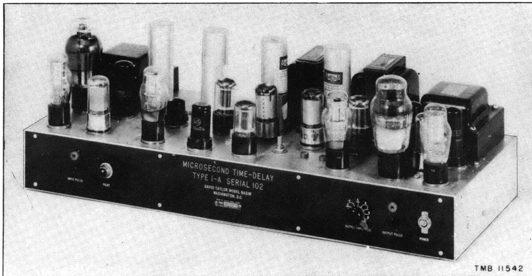
Figure 7 - Microsecond Time-Delay Unit View from the front with the chassis-protecting hood removed.
