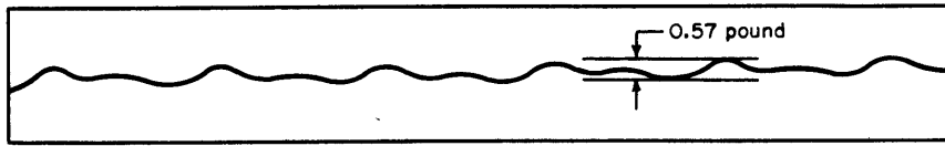
Figure 20a - Drag under Load Imposed by 50-Pound Weight Towed from Forward Towpoint Average drag, 27.90 pounds; Towing speed, 10.02 knots; Frequency, 1.14 cycles per second.
