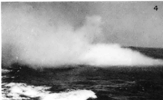
Figure 12 - Growth of a Dome and Plumes from an Underwater Explosion The phenomenon is partially obscured by smoke from the ship from which the photographs were taken.
