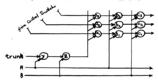
The driving lines A and B are alternately pulsed with 0's. This will propagate a linserted at the beginning of the trunk line up to the core Z, where the propagated 1 will die if switch cores a1, a2, a3.... all contain O's. However, if previously the control switch has inserted a l in one of the switch cores, the 1 will continue to be propagated down the channel headed by that core, and no other.
