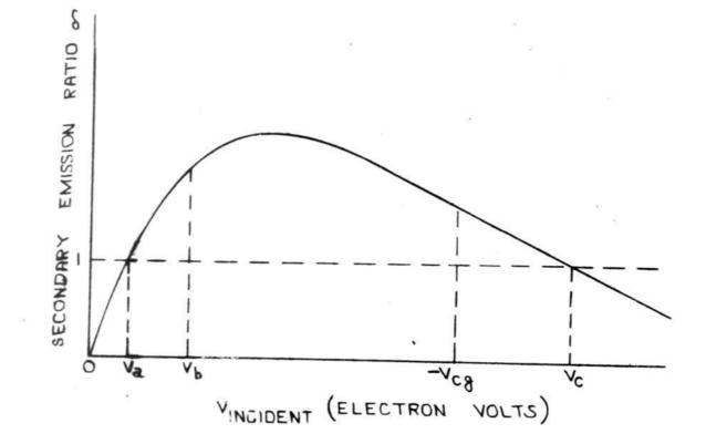
FIG. 19 SECONDARY EMISSION RATIO AS A FUNCTION OF THE ENERGY OF INCIDENT PRIMARY ELECTRONS.
