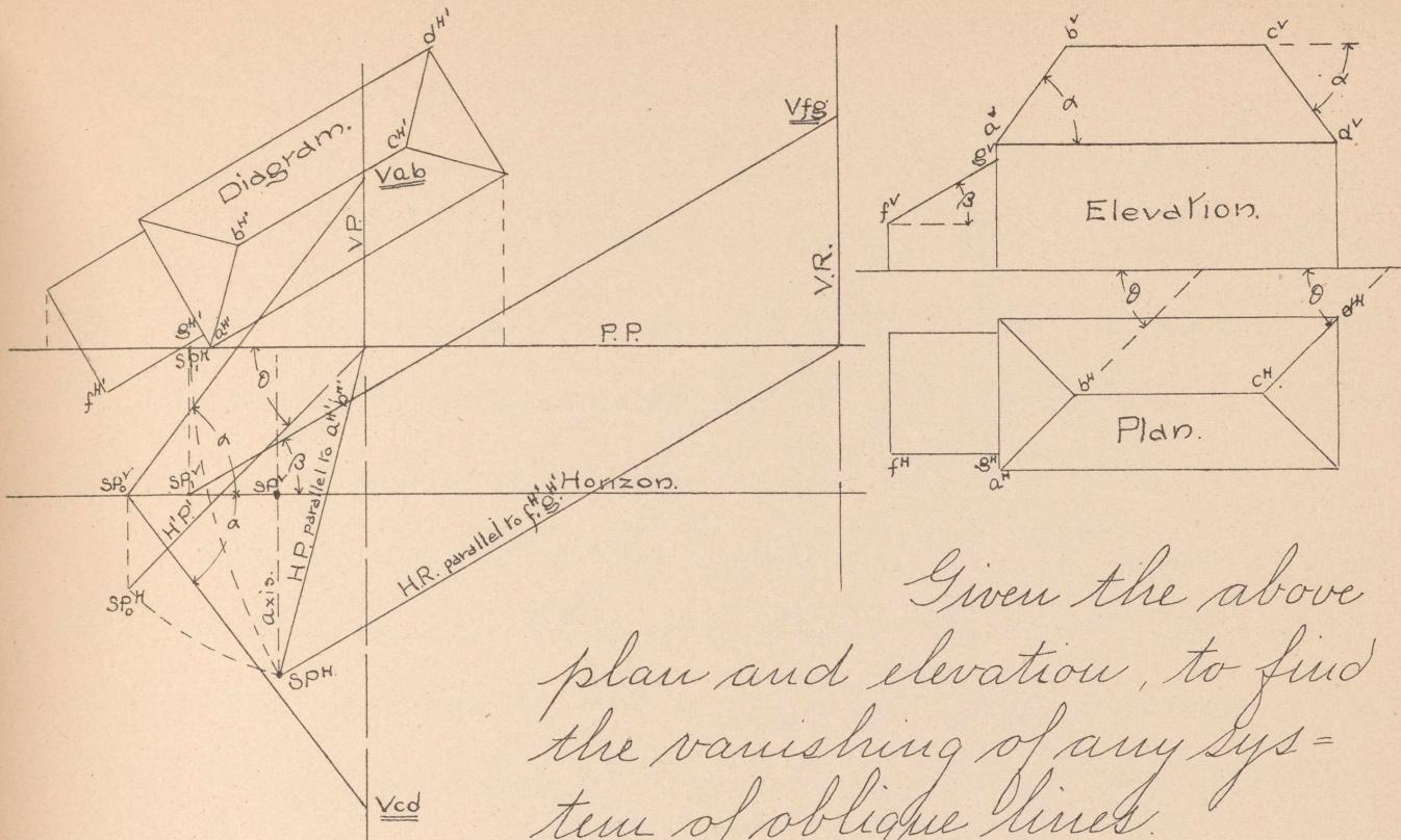
Given the above plan and elevation, to find the vanishing of any system of oblique lines.
