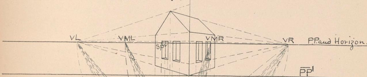
The point (a) may be assumed anywhere on  $\overline{P''P}$ , between vertical lines dropped from VR and VL.
