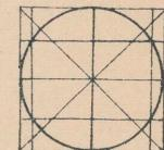
(27) When the P.P. is taken parallel to one of the systems of horizontal lines, the result is one-point or parallel perspective. This is generally the case in interior perspective. The axis in order to give a better effect is, in this case, often assumed to one side or the other of the center. If the method of finding vanishing points is applied to this case, it will be seen that VR, VL, and  $\overline{SPY}$  coincide.
