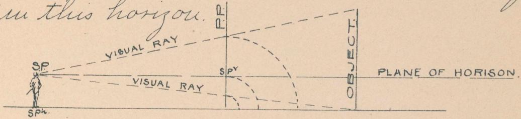
(9) A perspective drawing is the projection of an object upon a plane surface called the Perspective Plane, or the Picture Plane (P.P.) This takes the place of the vertical plane in ordinary projections. The position of the eye of the observer is called the Station Point. (S.P.)
