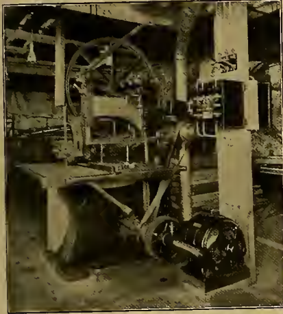
FIG. 1. INDUCTION MOTOR DRIVING BAND SAW IN PIANO FACTORY
