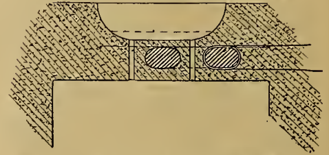
Fig. 1. Cross-section of Mold and Heating Coil USE OF ELECTRIC HEAT IN MAKING CASTINGS
