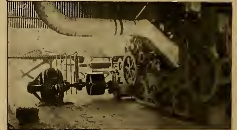
FIG. 5. TIMBER SIZER DIRECT-CONNECTED TO 55-HORSEPOWER INDUCTION MOTOR
