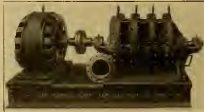
TURBINE PUMP DIRECT-CONNECTED TO INDUCTION MOTOR
