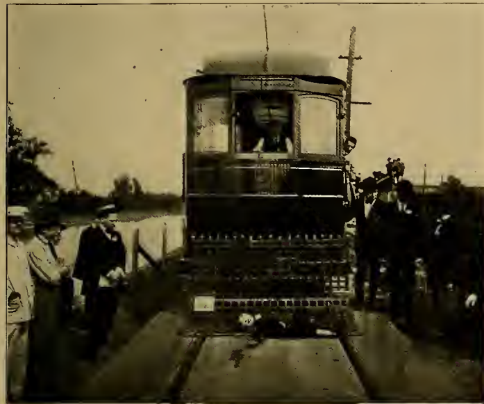
Boy Dummy Picked Up by O'Leary Fender on Asphalt-paved Track
