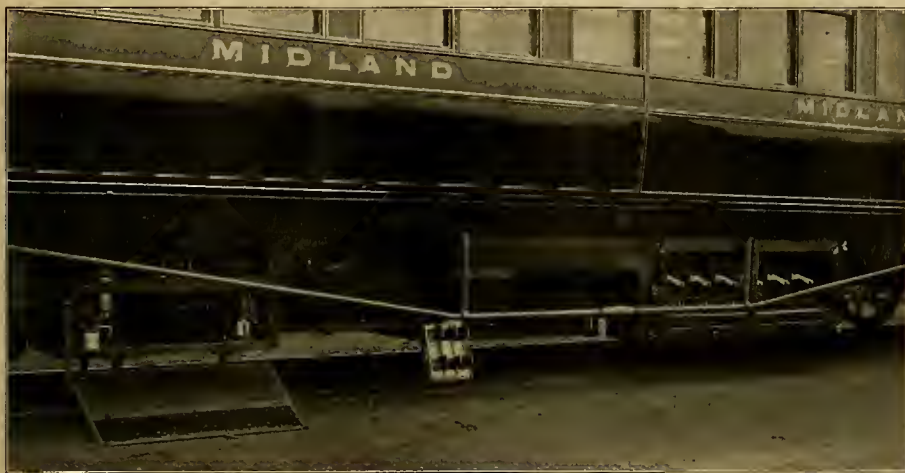
High-tension and Contactor Chambers are Shown Open. UNDERFRAME OF SIEMENS CAR USED ON FIRST SINGLE-PHASE RAILWAY IN ENGLAND.
