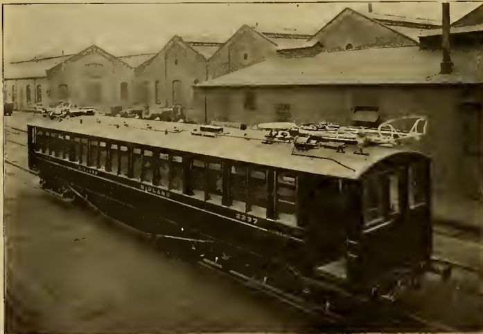
Siemens Car, Showing Bow Contacts.
