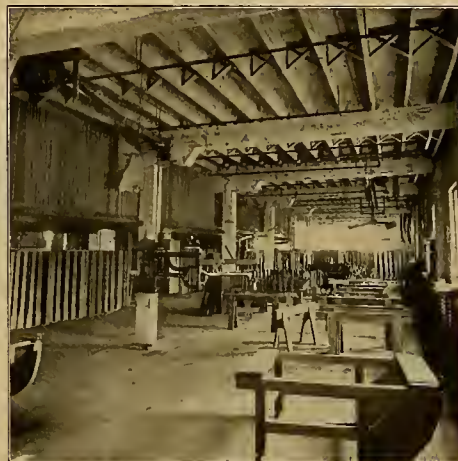
FIG. 3. CEILING MOTORS DRIVING BORING MACHINES
