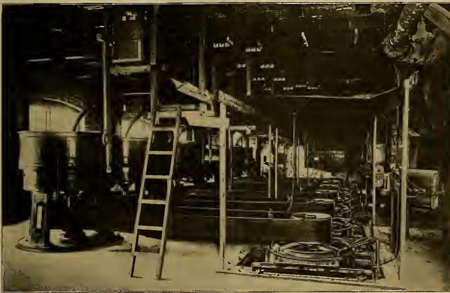
VERTICAL 75-HORSEPOWER INDUCTION MOTORS BELTED TO BUHR MILLS IN GLUCOSE FACTORY.
