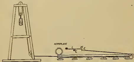
FIG. 16. STARTING MECHANISM OF THE AEROPLANE
