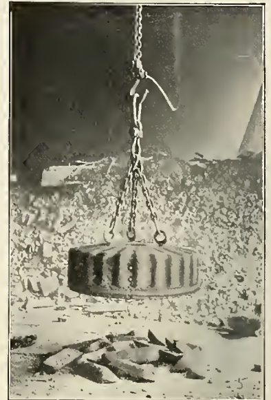
HANDLING MACHINE-CAST PIGS WITH LIFTING MAGNET.
