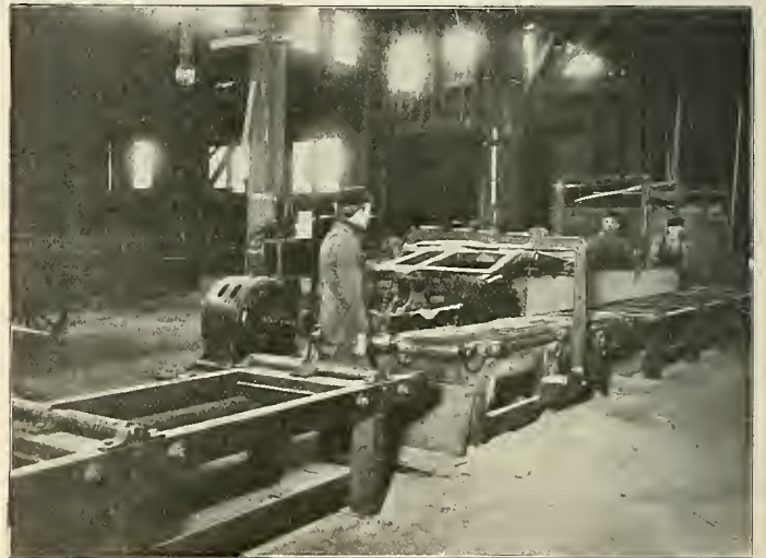
This saw will rip a timber 12 inches square and 12 feet long in one minute. 48-INCH SAW DIRECT-CONNECTED TO 40-HORSEPOWER MOTOR.
