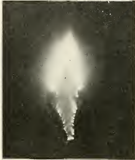
FIG. 2. ELECTRIC FLAME FROM DIVERGING ELECTRODES USED IN PRODUCTION OF NITRIGENOUS COMPOUNDS.
