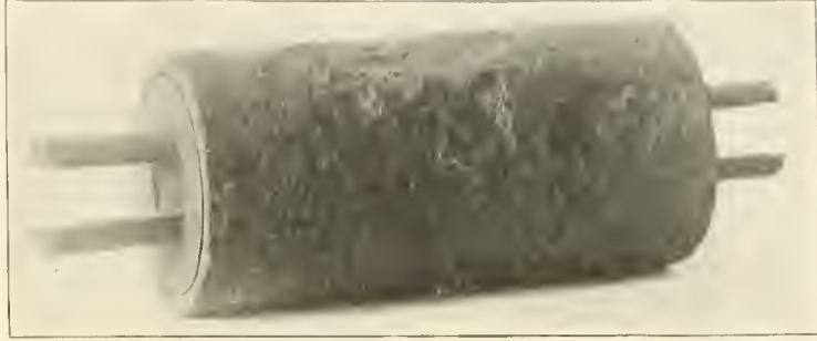
A PIECE OF THE FIRST UNDERGROUND ELECTRIC-LIGHT CABLE (NATURAL SIZE) LAID IN CHICAGO.
