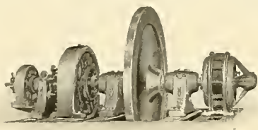
FIG. 3. MOTOR-GENERATOR SET WITH FLYWHEEL.
