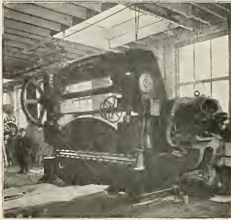
A 15-HORSEPOWER MOTOR DRIVING FORMING PRESS IN SHEET-METAL WORKS.
